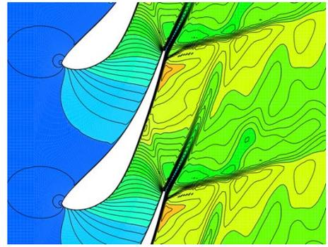
Instantaneous Mach number contour plot at 50% span location
