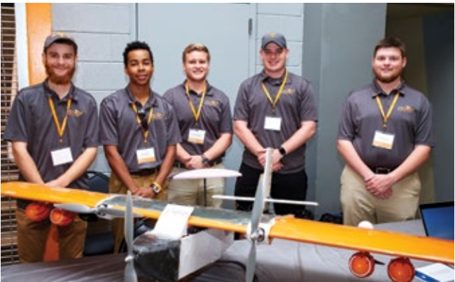
The AIAA design, build, fly team designed and built a remote-controlled aircraft capable of simulating aircraft carrier operations.
