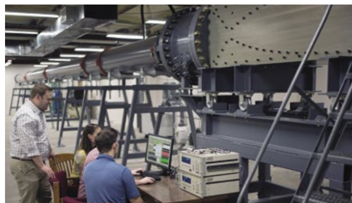
One of the largest wind tunnels in use in academia is housed at UTSI.
